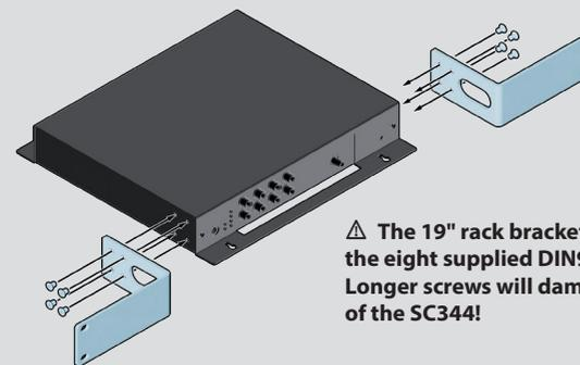
⚠ The 19" rack brackets must be fixed with the eight supplied DIN965 M4x6 screws. Longer screws will damage the electronics of the SC344!
